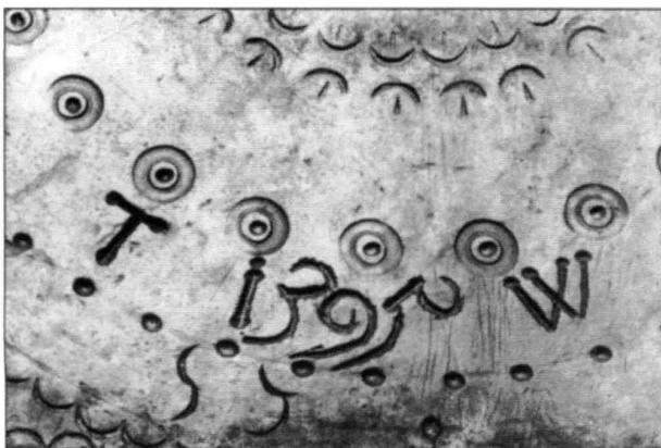
Fig. 5: Close-up photograph showing the detail of the punched initials 'T' / 'W' and the numerals '1395' chiselled into the underside of the dial-plate. The initials may be those of the original maker, diallist, or patron. The date is probably an error that caused the instrument to be reversed and engraved on the other side.
